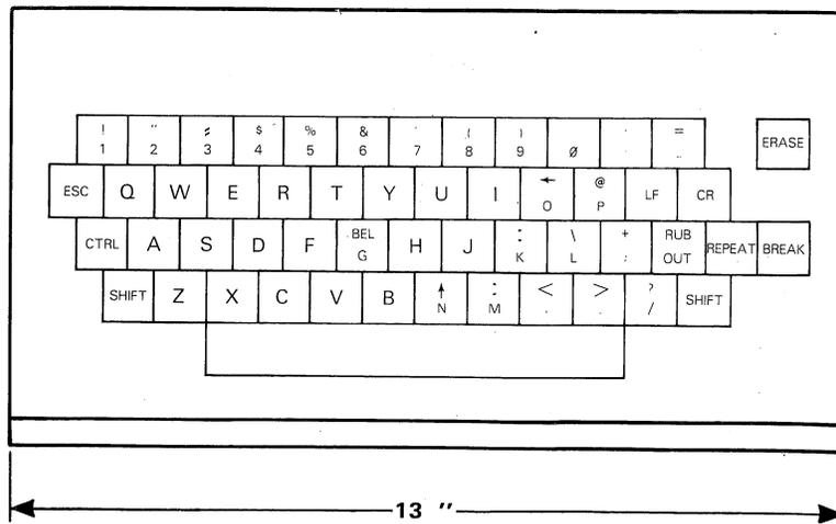
FIGURE 29 DIMENSIONS, MODEL 440 KEYBOARD
