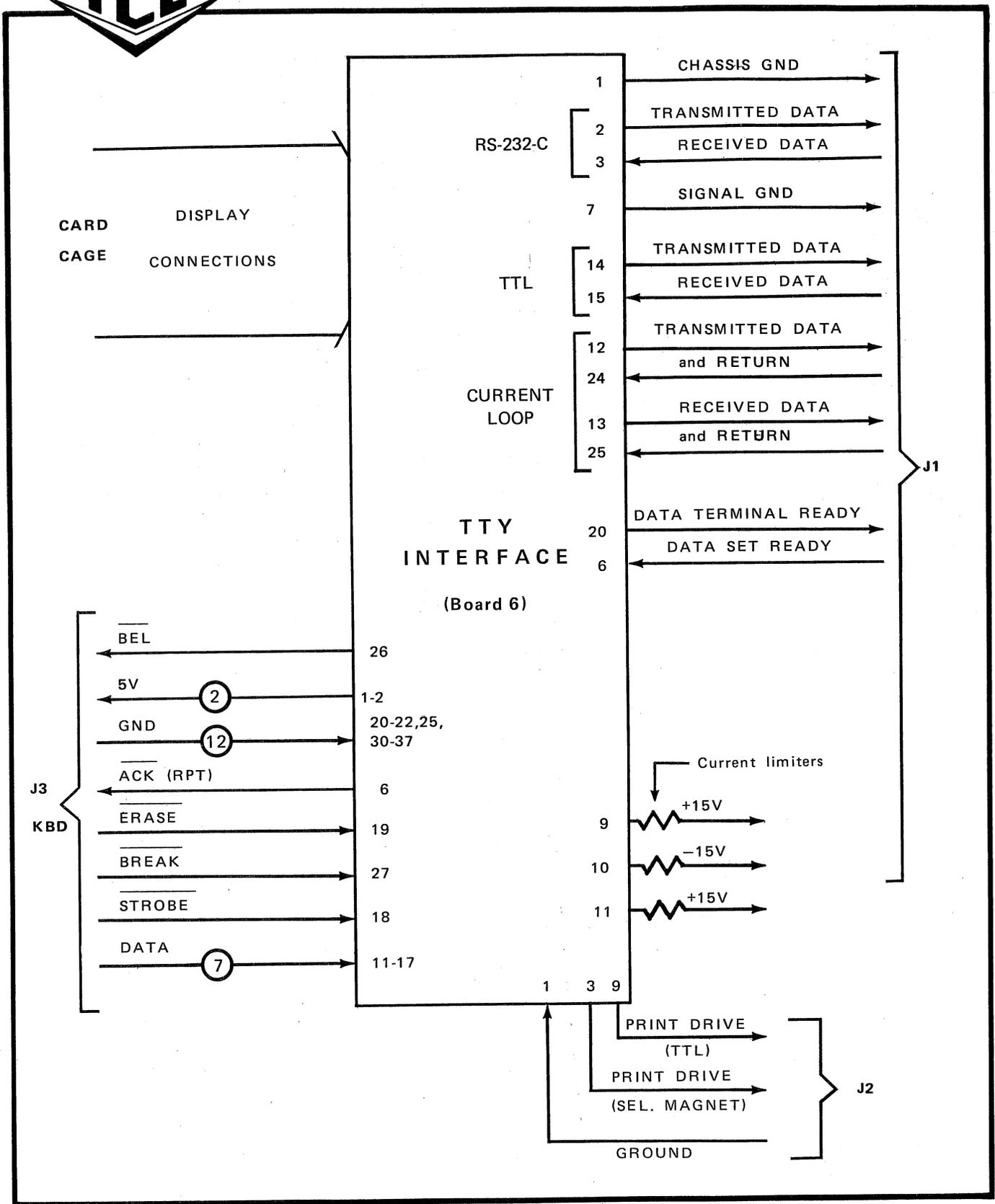
FIGURE 15 MODEL 440 TTY INTERFACE CONNECTIONS
