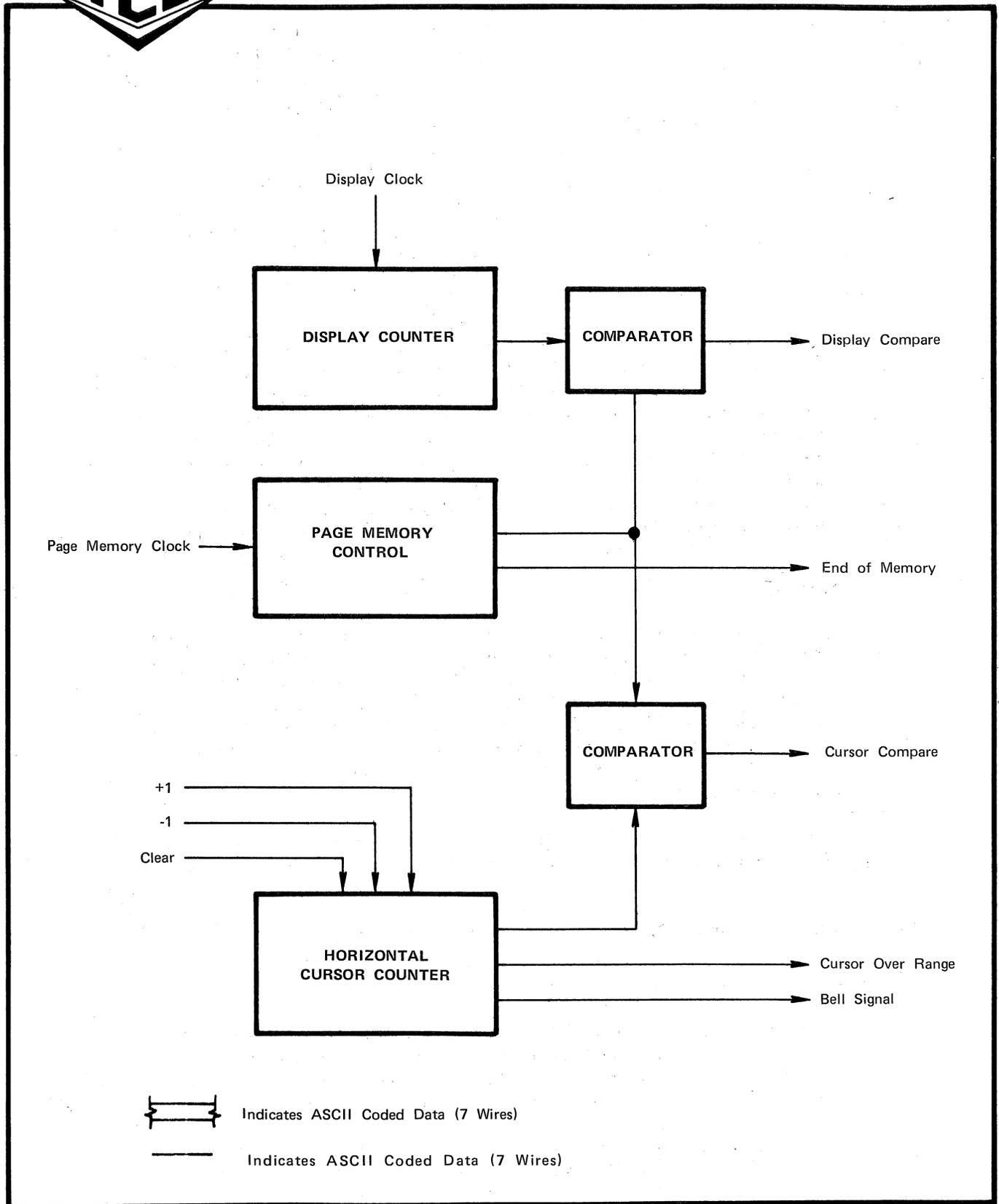
FIGURE 11 FUNCTIONAL DIAGRAM – PAGE CONTROL
