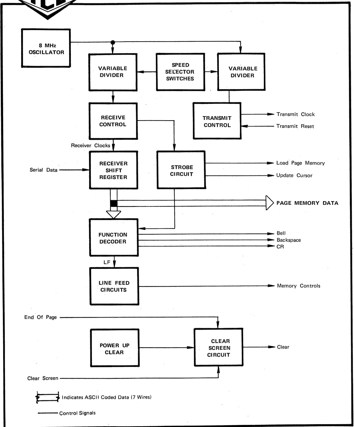
FIGURE 12 FUNCTIONAL DIAGRAM – FUNCTION CONTROL
