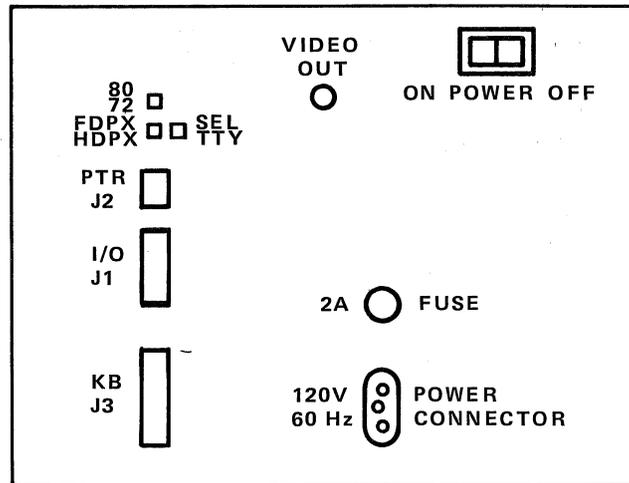
FIGURE 5 BACK PANEL CONNECTOR AND SWITCH LOCATIONS
