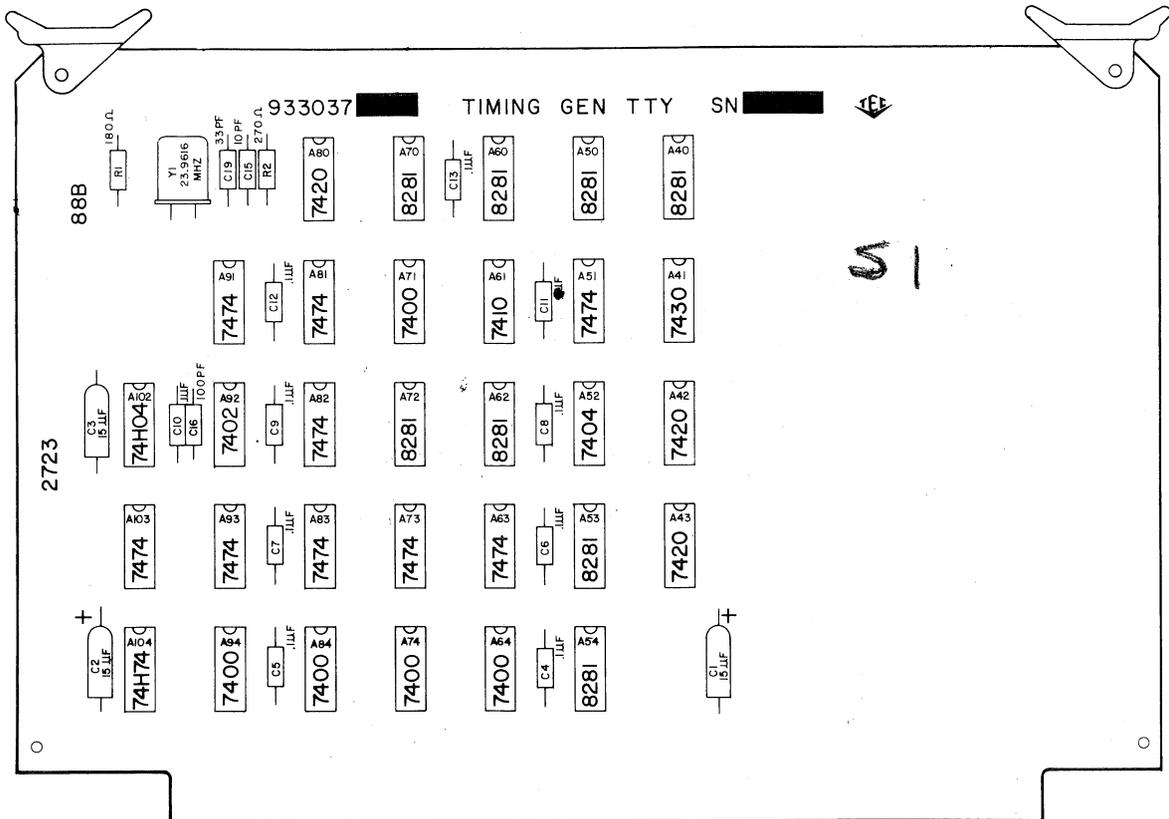
FIGURE 20 MODEL 440 TIMING GENERATOR PRINTED CIRCUIT BOARD
