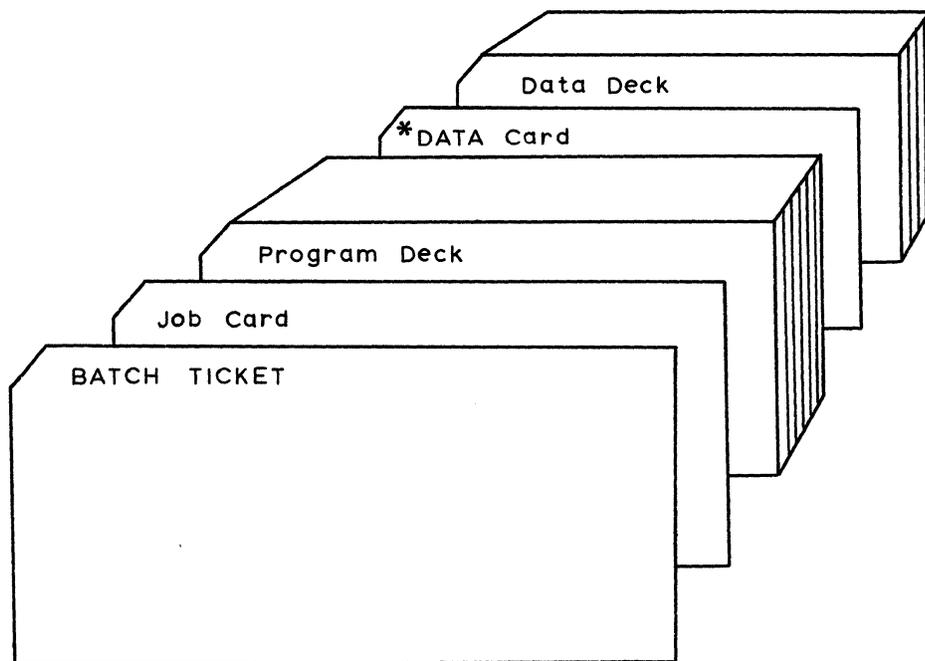
Figure 2. Structure of typical WATFIV deck for batch processed FORTRAN.
